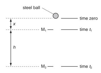
A steel ball is released at time zero from a point a distance x above M<sub>1</sub>. The ball reaches M<sub>1</sub> at time  $t_1$  and reaches  $M_2$  at time  $t_2$ . The acceleration of the ball is constant.
