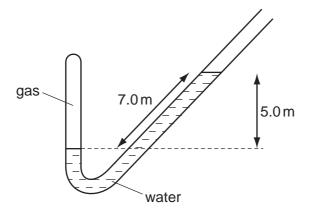
The atmospheric pressure is  $1.0 \times 10^5 \, \text{Pa}$ . The density of water is  $1000 \, \text{kg m}^{-3}$ .
